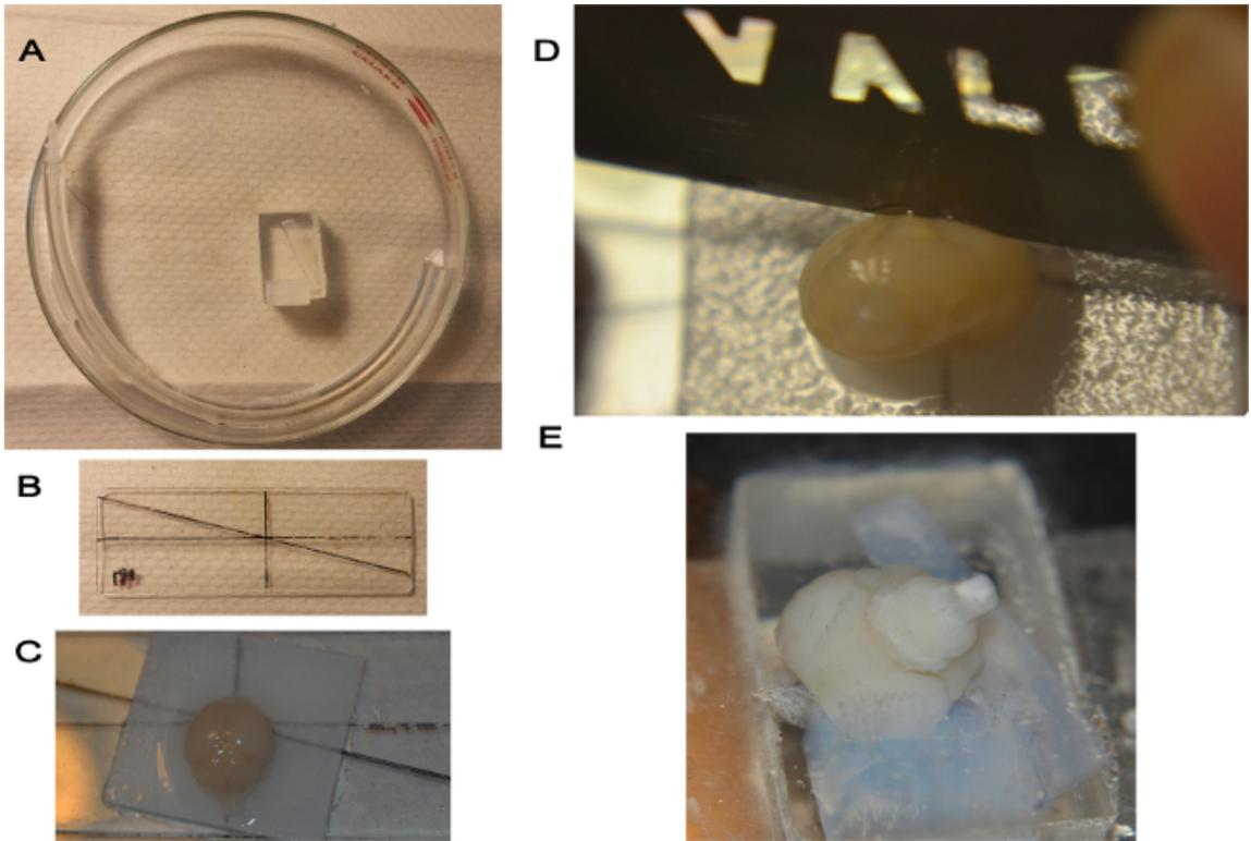
**Figure 2. Cutting the brain for slicing.** (A) Agar positioning on the cutting stage. (B) Slide for brain positioning. (C) Position of brain for anterior cut. (D) Position of brain and razor for double angled cut. (E) Final blocking of brain for slicing.
