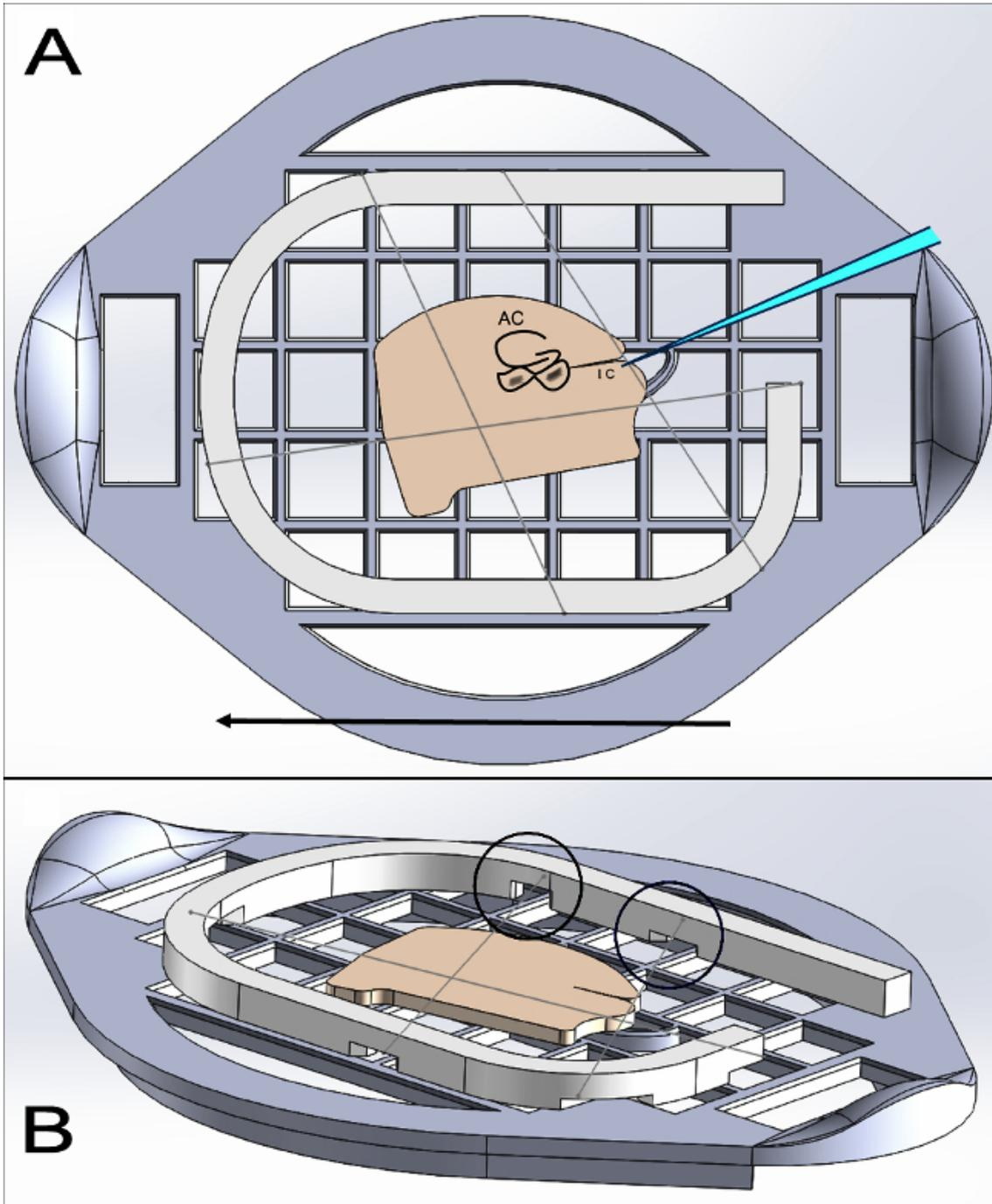
**Figure 1. Rendering of 3D printed materials. (A)** Rendered image of the slice sitting on the bridge with the printed harp in place. Arrow indicates flow of aCSF. **(B)** Rendered image highlighting grooves for the strings of the harp allowing for the thicker slice (circles).
